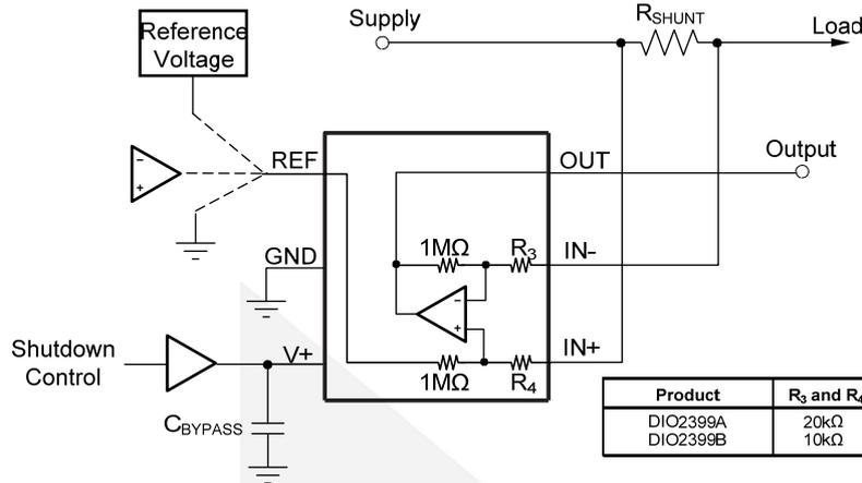
**Figure 13. Basic Circuit for Shutting Down DIO2399x with Grounded Reference**
