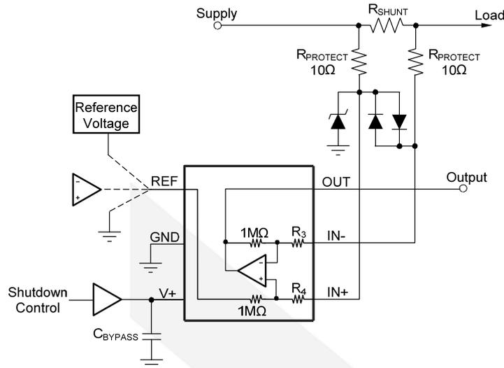
**Figure 16. DIO2399x Transient Protection Using a Single Transzorb and Input Clamps**
