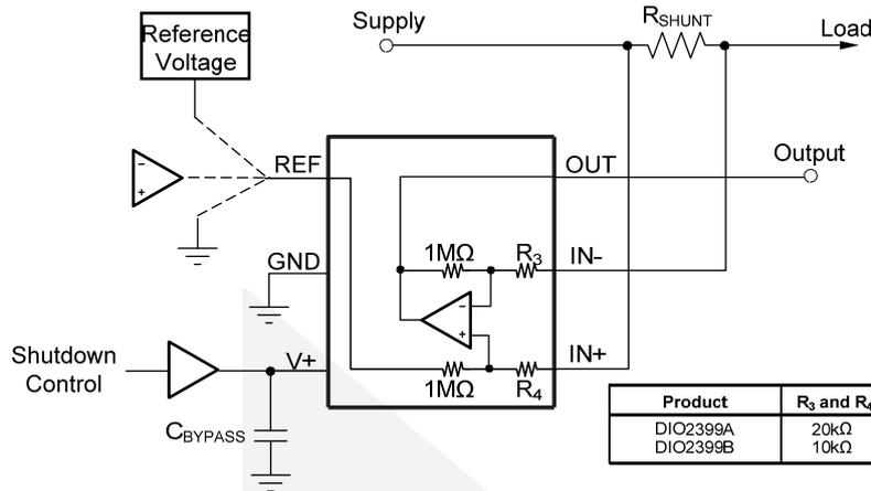
**Figure 13. Basic Circuit for Shutting Down DIO2399x with Grounded Reference**
