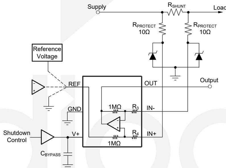
**Figure 15. DIO2399x Transient Protection Using Dual Zener Diodes**
