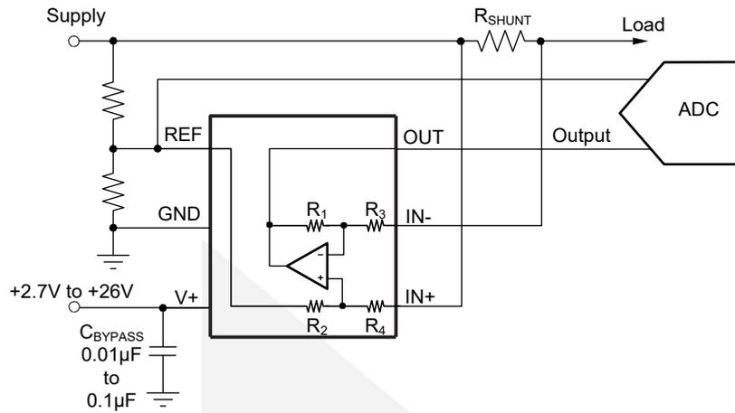
**Figure 14. Sensing DIO2399x to Cancel Effects of Impedance on the REF Input**
