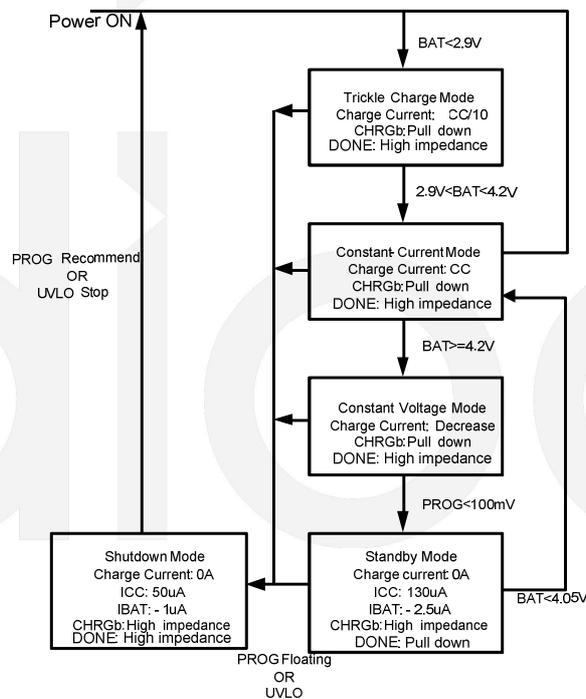
**Figure 4. State Diagram of a Typical Charge Cycle**
