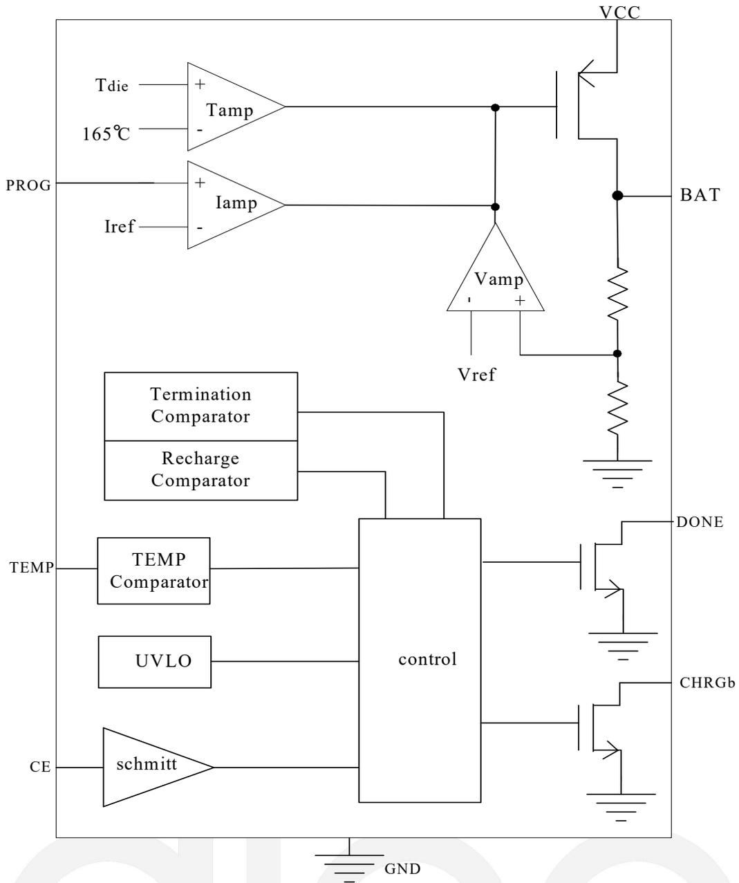
Figure 3 Block Diagram
