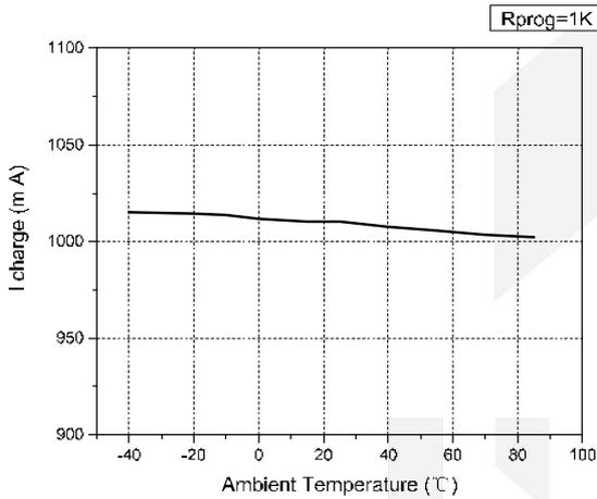
**I<sub>trickle charge</sub> vs. Ambient Temperature**
