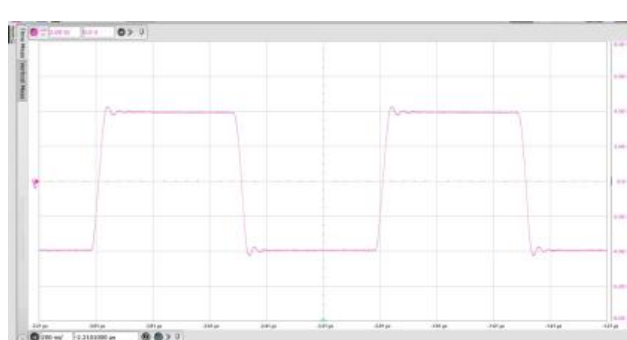
V_{CC} = 10\text{ V} , V_{OUT} = 8\text{ V}_{PP} , G = -1 Figure 17. Large signal step response
