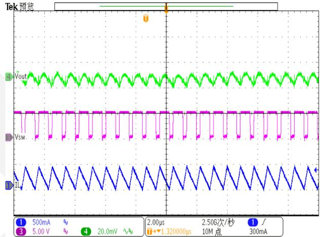
Vin=3.7V, Load=50mA start up by Vin
