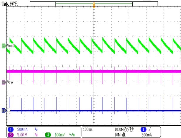
Vin=3.7V, Load=100mA at Heavy Load
