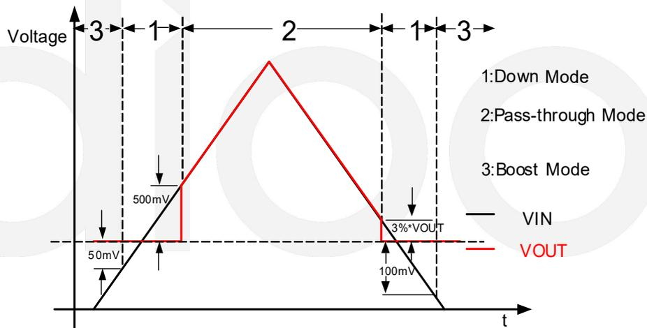
Figure 2 Down Mode and Pass-Through Operation
